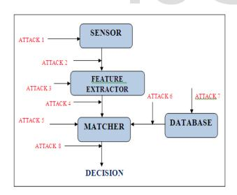
ATTACK 1 A fake biometric trait such as an artificial Finger may be presented at the sensor. In this case no A detailed system knowledge or access privilege is necessary.
